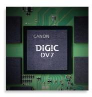
The newly developed DIGIC DV7 image processor boasting high data processing power while suppressing noise has been adopted.
